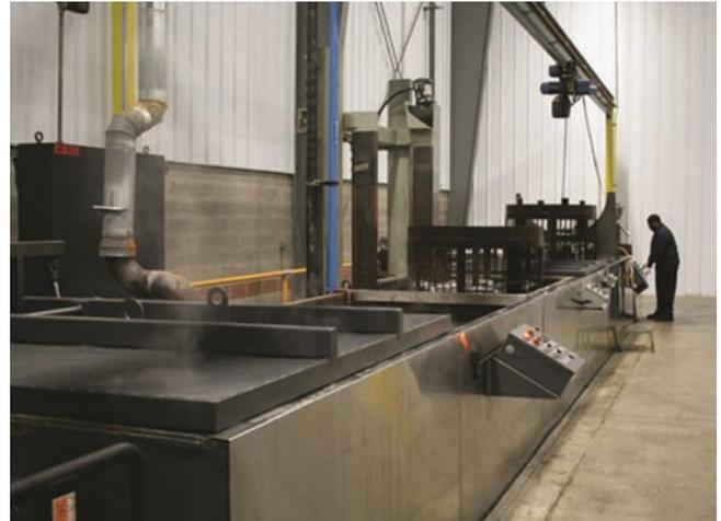
Figure 1 – Batch Process Vacuum Impregnation System.
